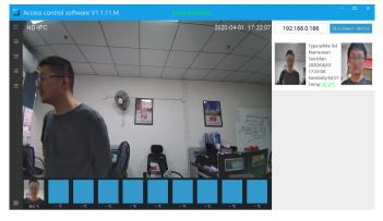
3. Recognition matching result information display window: When the captured face matches the face database in the device, it will be displayed here. It can display the face recognition similarity, temperature and other information. If there is no matching information in the face database, it will not be displayed.
